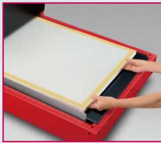
1. Set a screen stretched onto a frame
